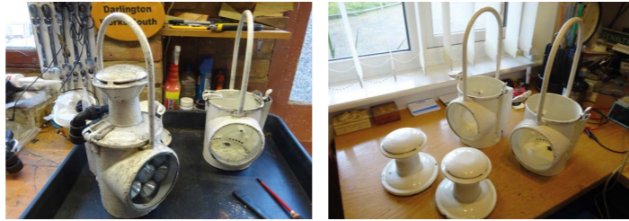
Above left: The two in-service headlamps after a year on the front of the loco, looking forward to their annual refresh, and right, headlamp bodies cleaned and repainted.
