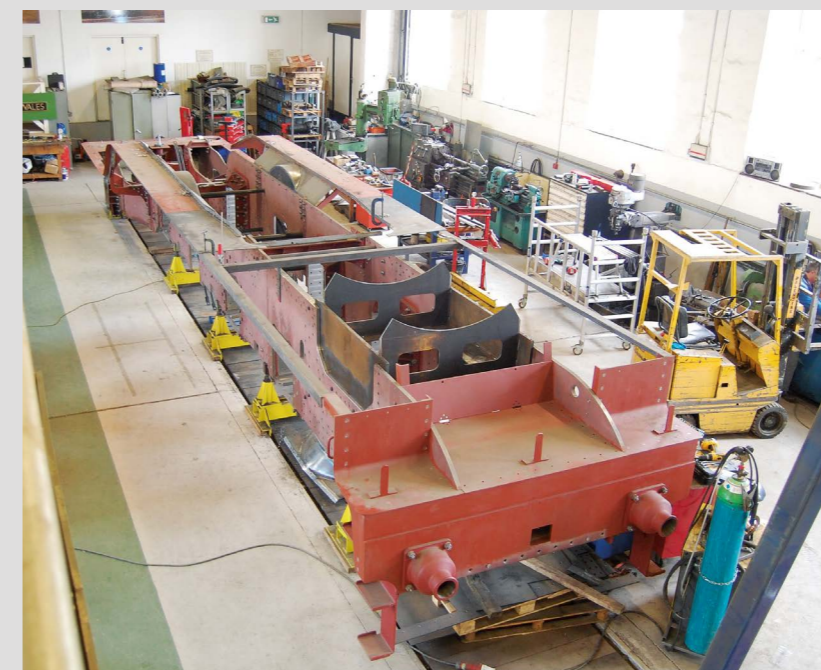
No. 2007's frames, Spring 2021 with temporary smokebox saddle stay and right, the welded smokebox.
