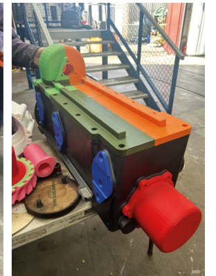
Above: (from left to right) - A pile of full-size printed valve and cambox parts, the cambox with its lid off showing the camshaft in place, then two images showing the assembled cambox.
