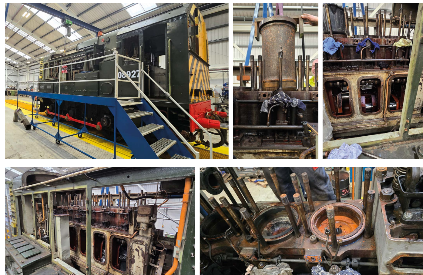
Above: A selection of images showing the work involved in getting the 08 back into service.
