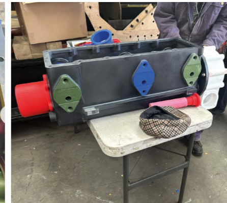
Above: (from left to right) - A pile of full-size printed valve and cambox parts, the cambox with its lid off showing the camshaft in place, then two images showing the assembled cambox.
