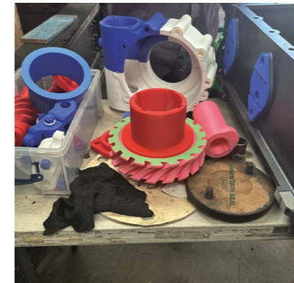
Above: (from left to right) - A pile of full-size printed valve and cambox parts, the cambox with its lid off showing the camshaft in place, then two images showing the assembled cambox.
