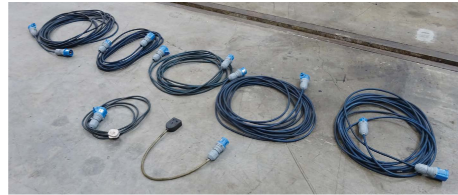
Above: Some of the coach shore power cables, fitted with new 16A connectors.
