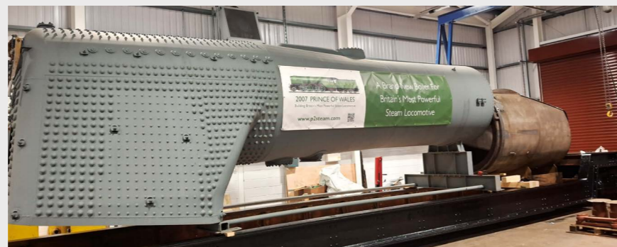
No. 2007's boiler in DLW.
