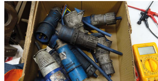
Above: Some of the coach shore power cables, fitted with new 16A connectors.
